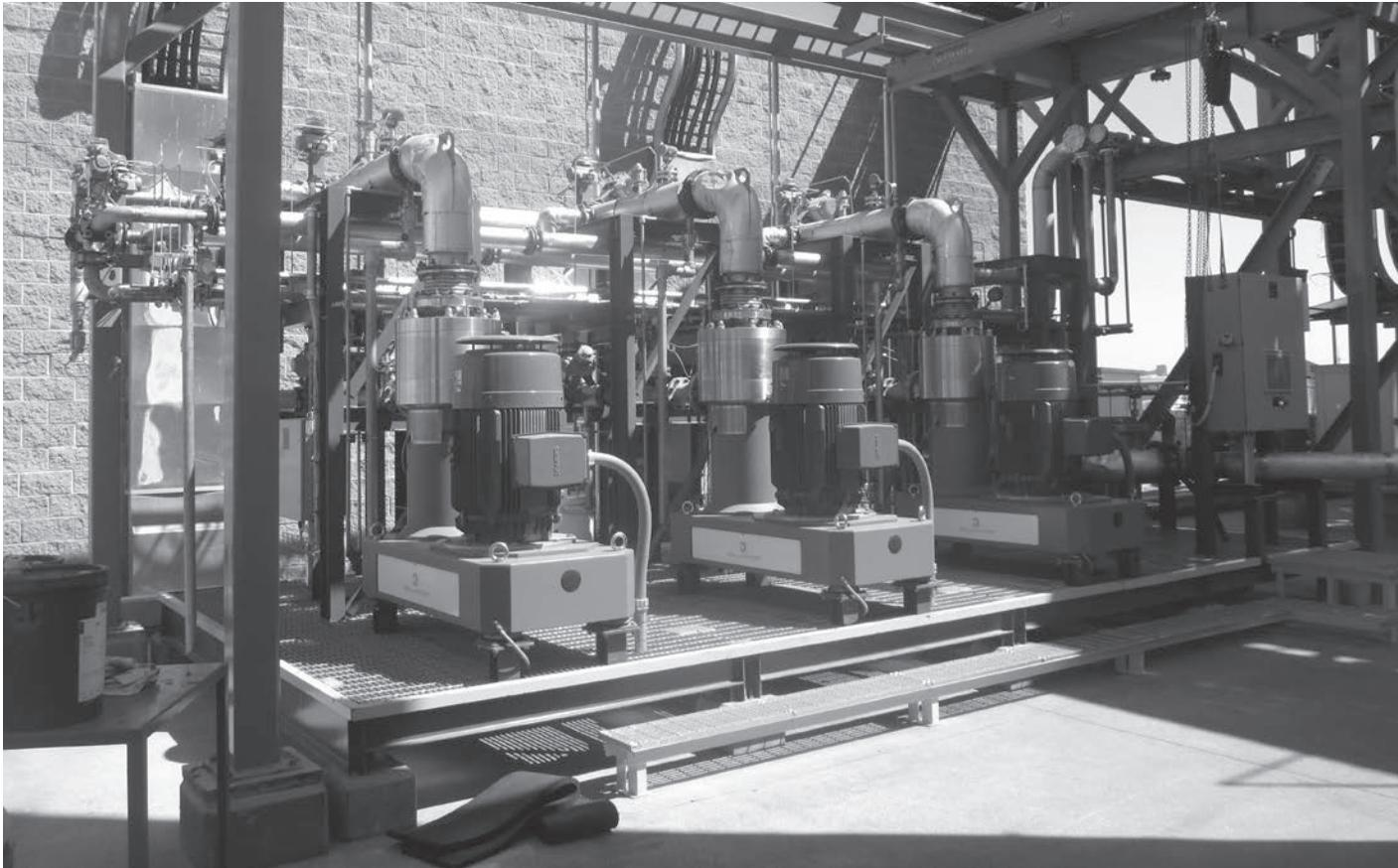
Contributed | Edeniq's proprietary Pathway Technology utilizes high-shear milling equipment called a Cellunator to convert corn-kernel fiber, a by-product of corn-based ethanol production, into cellulosic ethanol.
